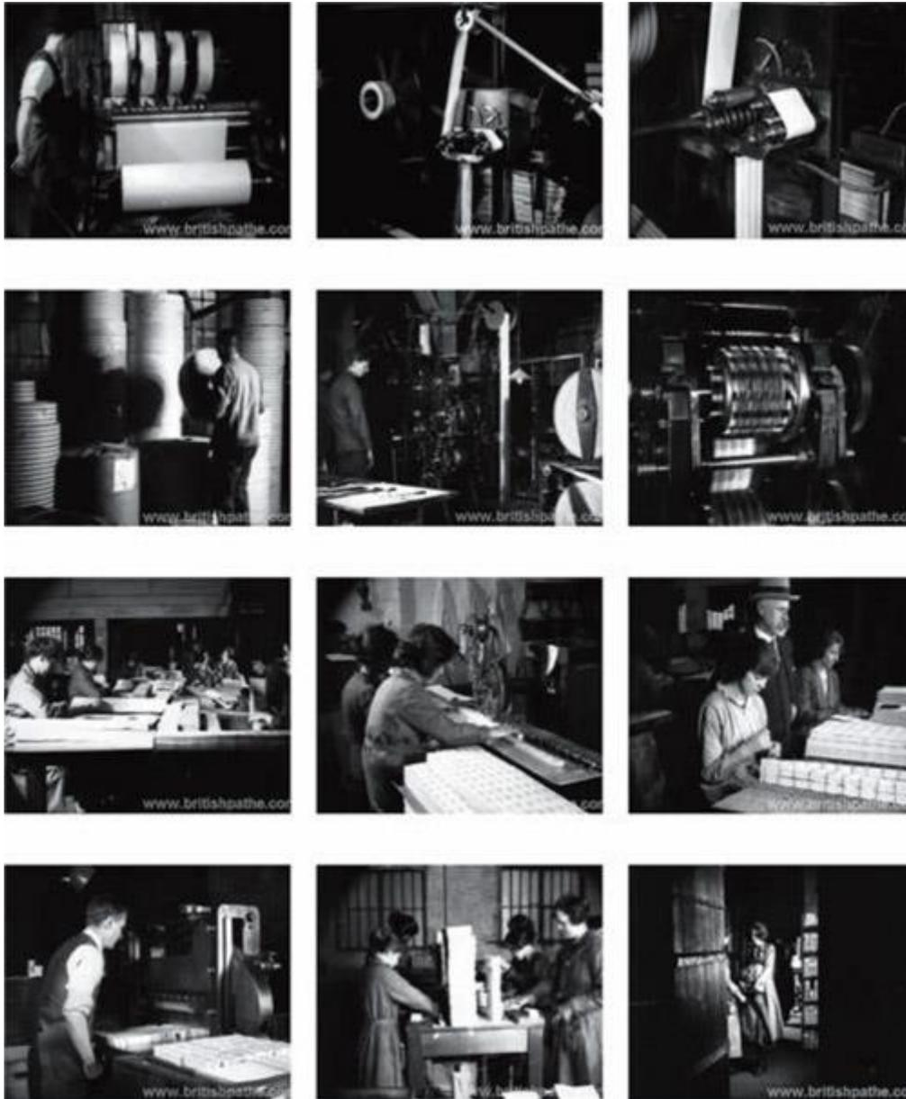
Short film showing tram tickets being produced: 1–3 a ream of paper is cut down into rolls, to which coloured dye is added; 4 the rolls are stacked ready for printing; 5–6 numbered tickets being printed with a special printing machine; 7–9 strips of tickets are sorted, wired, and then tied with string; 10–12 finally the tickets are guillotined, stacked, and stored on shelves before being delivered.
