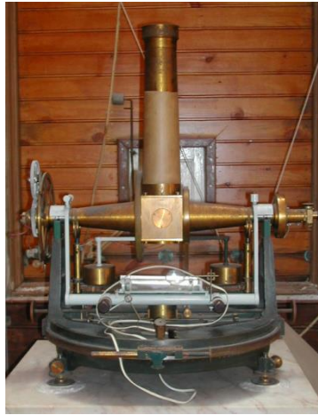
Fig. 11 – Portable transit instrument designed by Frederico Augusto Oom. (Observatory of Lisbon - MUNHAC)
